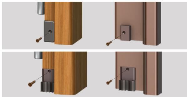
**BUTTON (F):** hexagonal brass, square nylon, bevelled nylon, rolling nylon (pivot).
